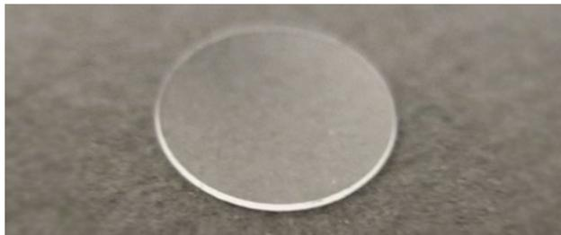
Figure 2: Macro camera photo of 5 mm disk cut from a 150  $\mu\text{m}$  thick sapphire wafer
