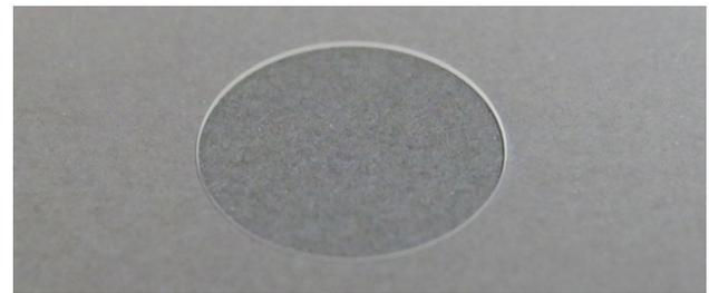
Figure 1: 10 mm diameter hole cut out in 200  $\mu$ m thick Corning Willow glass
