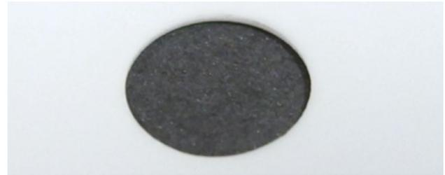
Figure 3: Digital camera photo of 5 mm diameter hole machined in 200  $\mu\text{m}$  thick alumina ceramic plate shows very good edge quality and no discoloration of the material.
